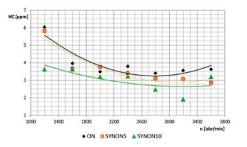
Fig. 7. Comparison of HC concentration in exhaust of AVL engine fuelled by mineral diesel fuel and mixtures of diesel fuel with synthetic hydrocarbons, working at full load
