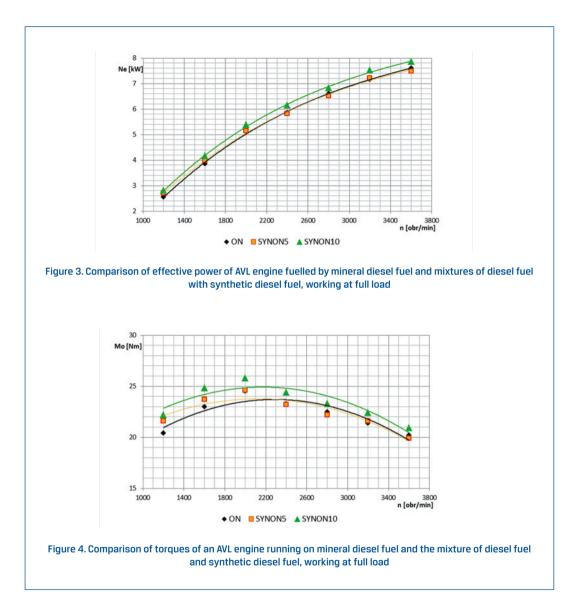
Values of CO,  $CO_2$ , HC,  $NO_x$  and  $SO_2$  in exhaust were registered at preparation of external performance specification. Recorded study results are presented below in form of diagrams. Fuel composition, in this case the addition of synthetic hydrocarbons, was found to have a considerable impact on emission level of particular components.
