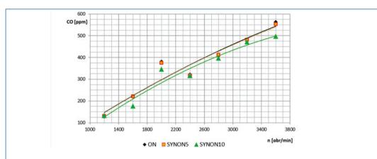
Fig. 6. Comparison of CO concentration in exhaust of AVL engine fuelled by mineral diesel fuel and mixtures of diesel fuel with synthetic hydrocarbons, working at full load
